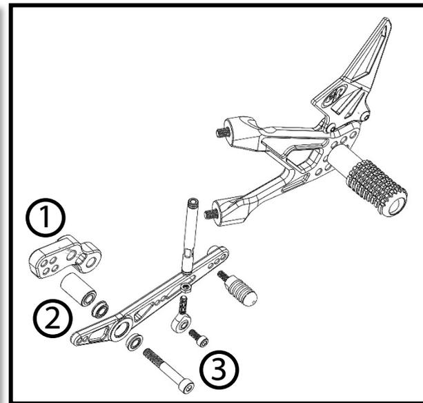
① The “kickstand delete” bracket is optional. Rearsets can be used with or without the kickstand with the appropriate components from us. Contact us if you’d like to switch from one arrangement to the other.
